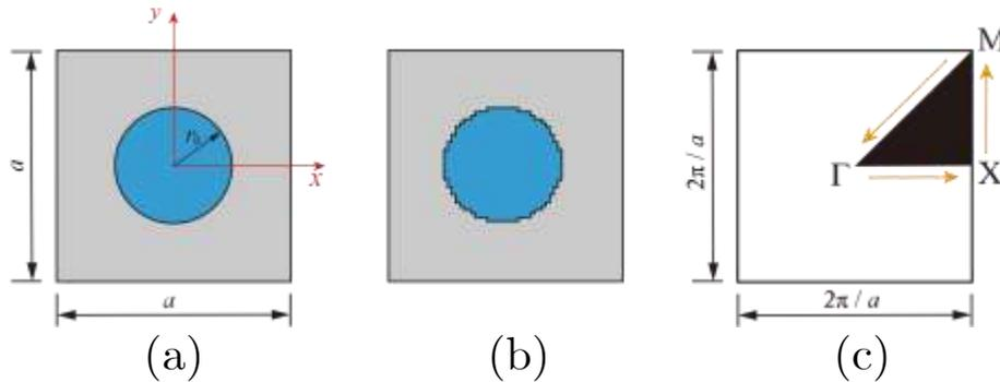
The 2-D two-phase phononic crystal with circular inclusions: (a) the unit cell, (b) rasterized unit cell, (c) the first irreducible Brillouin zone.
