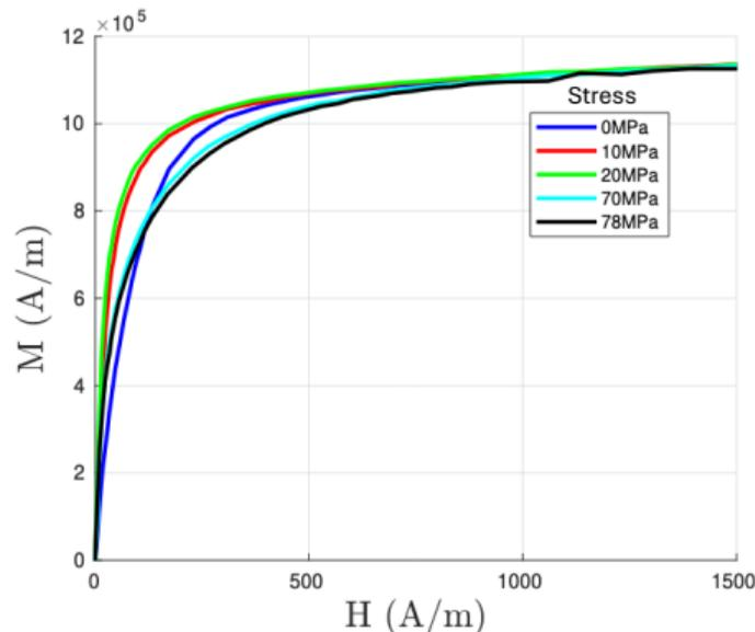
*Effect of uniaxial stress on magnetization behavior at constant stress, for non-oriented silicon-iron alloy*
