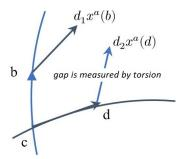
Dislocation density being interpreted to torsion tensor of a material connection
