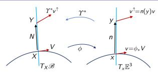
Let V be an arbitrary tangent vector to  $\mathscr{B}$  at a point  $X \in \mathscr{B}$ , the induced Ehresmann connection is naturally defined by considering its horizontal lift:
